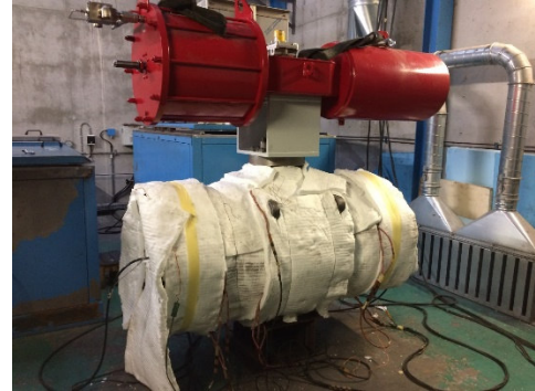
Figure 2: Axial Flow undergoing High temperature test.
