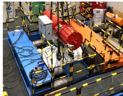
Figure 3: Axial Flow undergoing Shell Test
